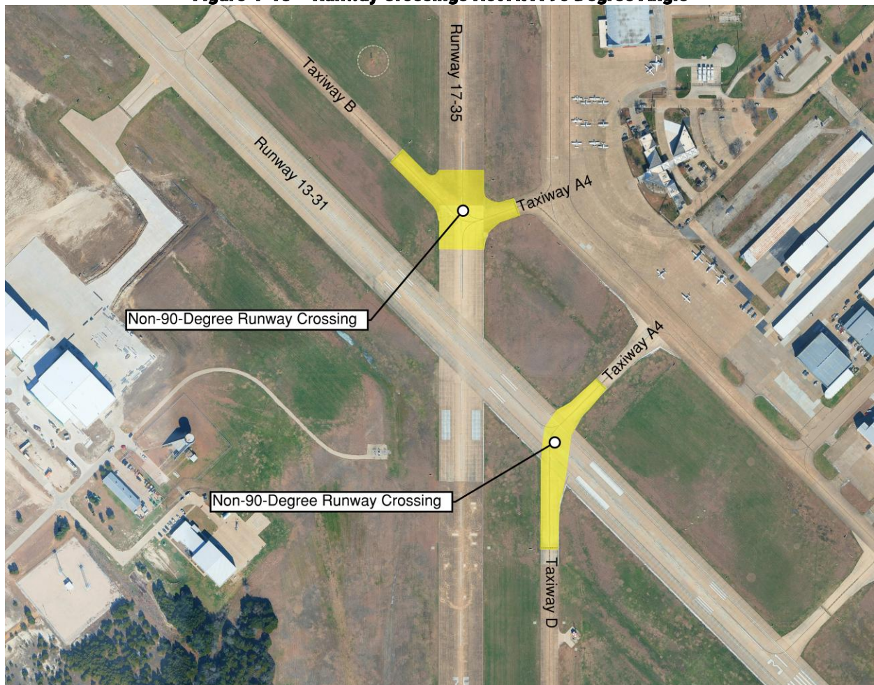
Figure 4-13 – Runway Crossings Not At A 90 Degree Angle
